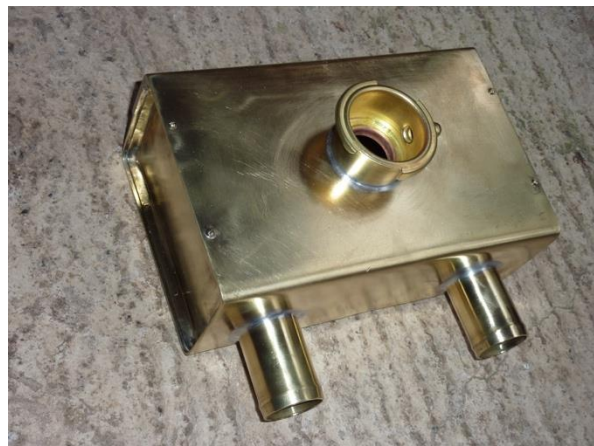
Bombproof header tank
