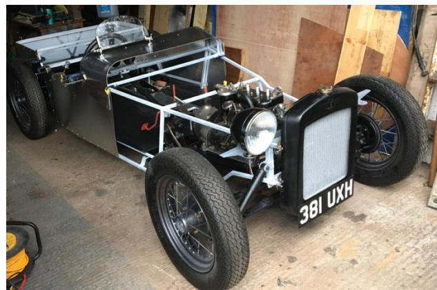
Frame and first panels on chassis
